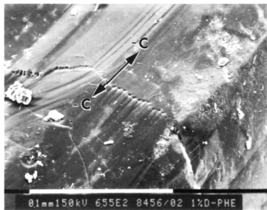
Figure 8. SEM photograph of the crack in a twinned ( R,S ) crystal. The c axis of the crystal is indicated.
